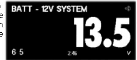
Each gauge can be displayed in two ways. The Graphic gauge shows the gauge value and two graphs. At the bottom of the screen is a simple bar graph indicating the current value. To the right is a histogram which shows how the value has fluctuated over the last minute. A flat graph indicates that the value is stable, and is not changing significantly.
