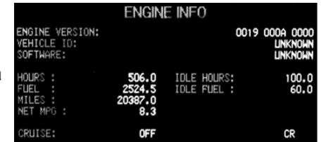
Included on this screen is data on the engine hours, fuel, miles, VIN, engine version, and idle time. These values are from the engine’s internal memory, and are accurate from the moment the engine was built, regardless of when the engine or VMS was installed. The miles value does meet the requirements as an odometer for reporting purposes when selling the vehicle.
