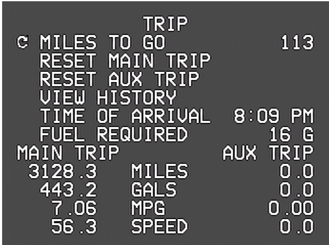
The first “Detail” screen displays information on your current trip. The unit tracks two trips simultaneously. You might use the main trip to track your mileage and fuel, say, each time you leave home, while the “auxiliary” trip keeps a cumulative total for the season or year, or you could reset it every time you refuel.
